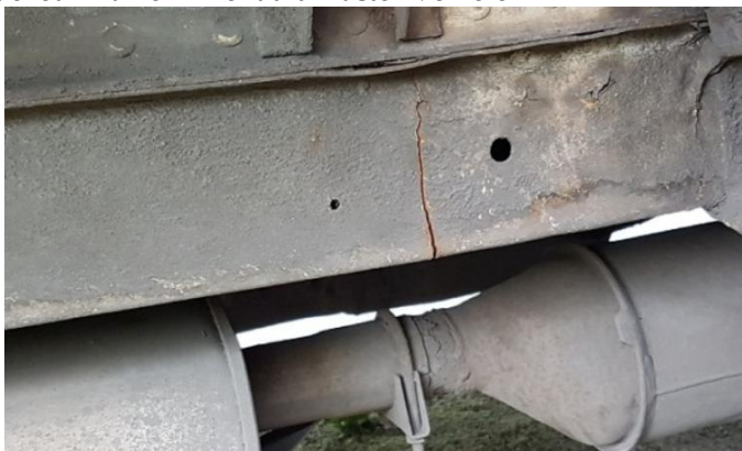
Figure 2. Cracked Frame in Renault Master Vehicle
