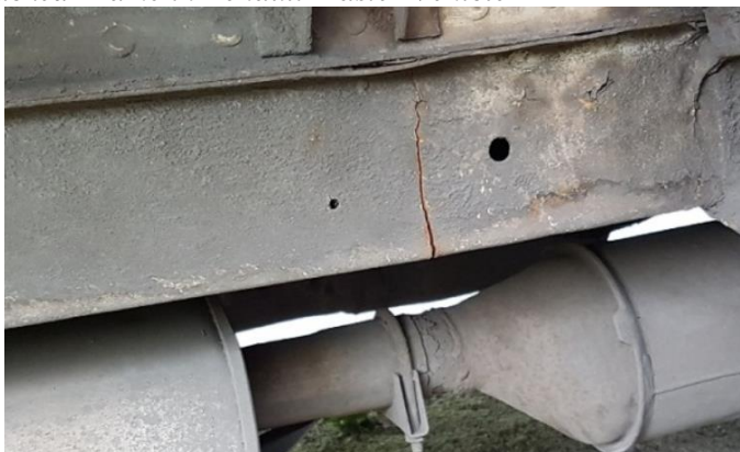
Figure 2. Cracked Frame in Renault Master Vehicle
